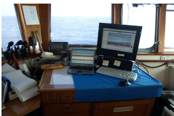
Figure 2. Top side monitoring station located on the bridge. Laptop (left) running Echoview and EK 60 topside PC unit (right).
