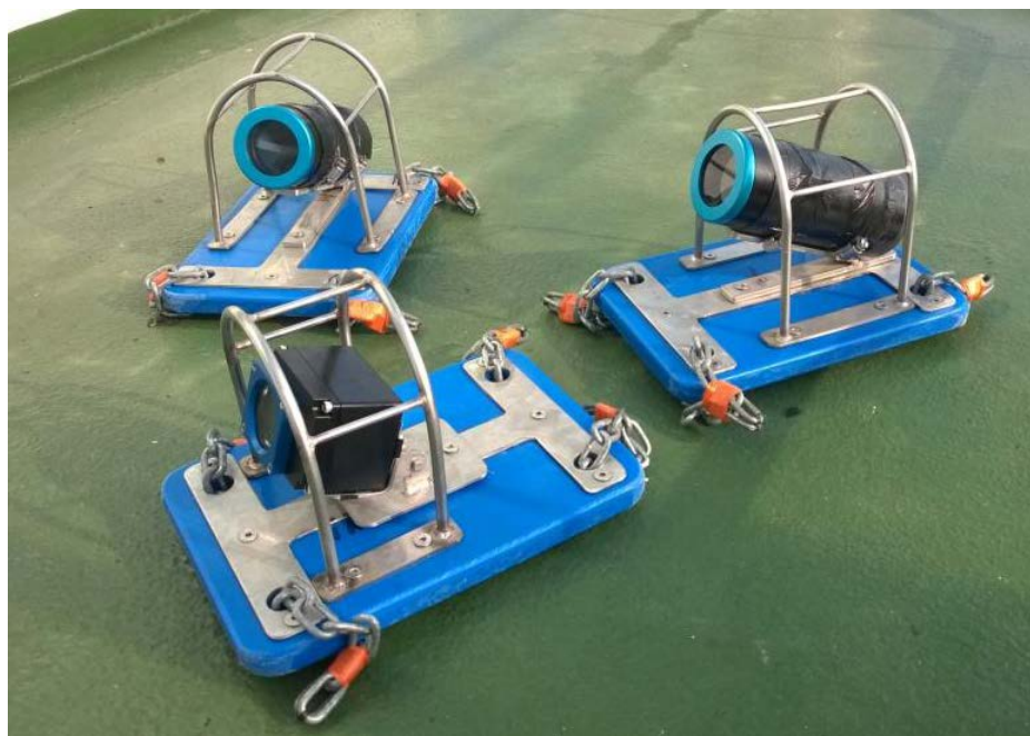
Figure 1 Camera (bottom) and lights on mounting plates.
