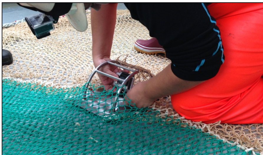
Photo 2. GoPro camera attached to inside of trawl by fish lock on Finnur Fríði IESSNS 2014. The steel frame was tied to trawl, at each corner using rope.
