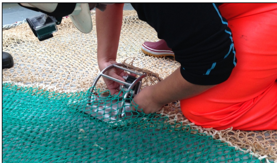
Photo 2. GoPro camera attached to inside of trawl by fish lock on Finnur Fríði IESSNS 2014. The steel frame was tied to trawl, at each corner using rope.
