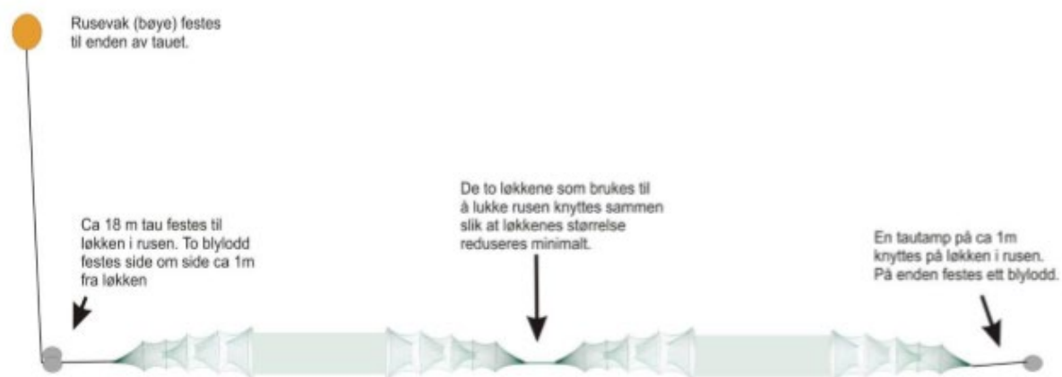
Figure 5. Double «eel» fyke net : From left; 1 fish chamber and 3 trunks, then guiding net, then 3 trunks and fish chamber. The second half mirrors the first. In total there are 4 fish chambers. (from van der Meeren, 2018).
