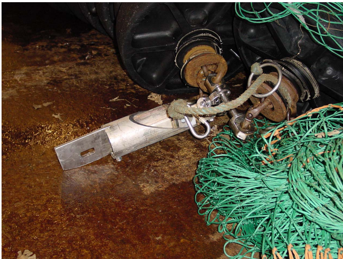
Figure 4.1. NOAA bottom contact sensor mounted on the footrope of a GOV trawl with C type ground gear.
