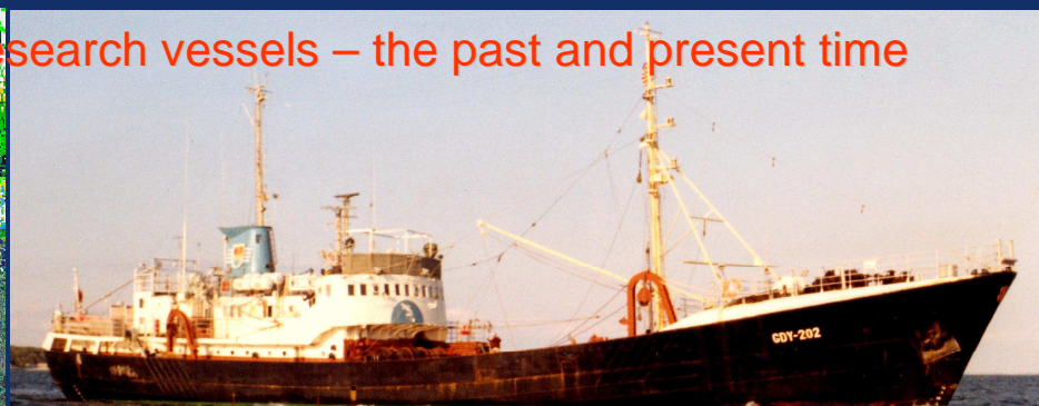
r/v „Wieczno” GDY-202, motor side-trawler type B-20, 61.4-m length and engine – 1375 HP, used in 1966-1989 for various surveys in the Atlantic and occasionally in the Baltic.
