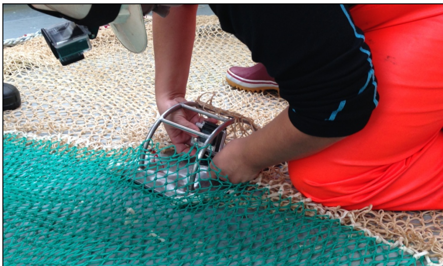
Photo 2. GoPro camera attached to inside of trawl by fish lock on Finnur Friði. The steel frame was tied to trawl, at the each corner using a rope.
