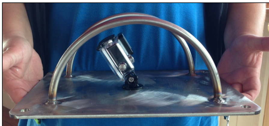
Photo 1. GoPro camera inside a waterproof box, mounted on steel frame and ready for employment in trawl on Finnur Friði.
