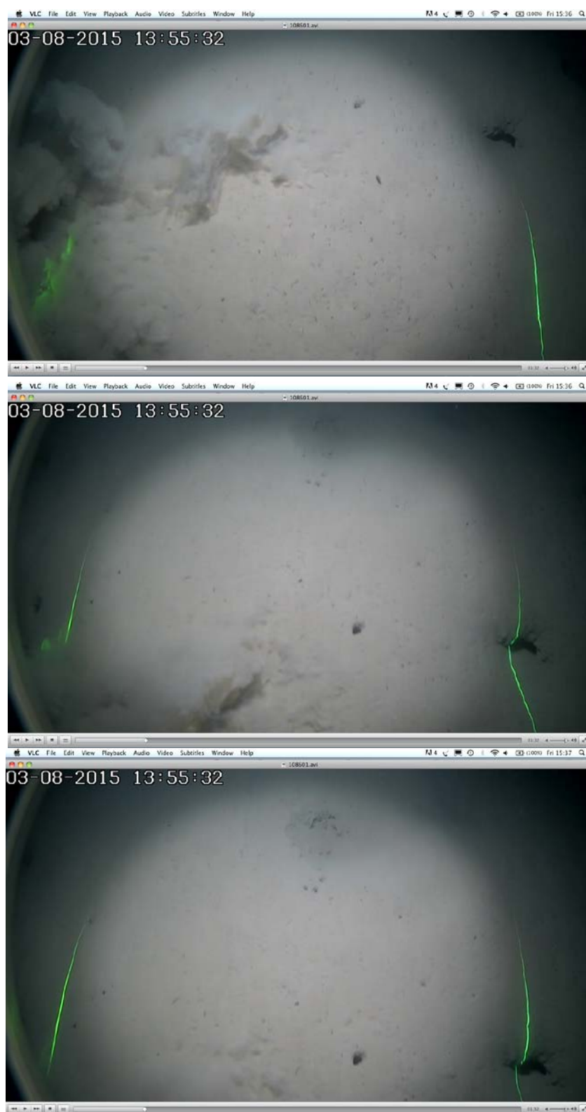
Figure 5.13. FU3-4: Still image of video footage showing the misinterpretation where the stripe laser appears to bend around burrows. In this case the burrow on the far right hand side is counted.
