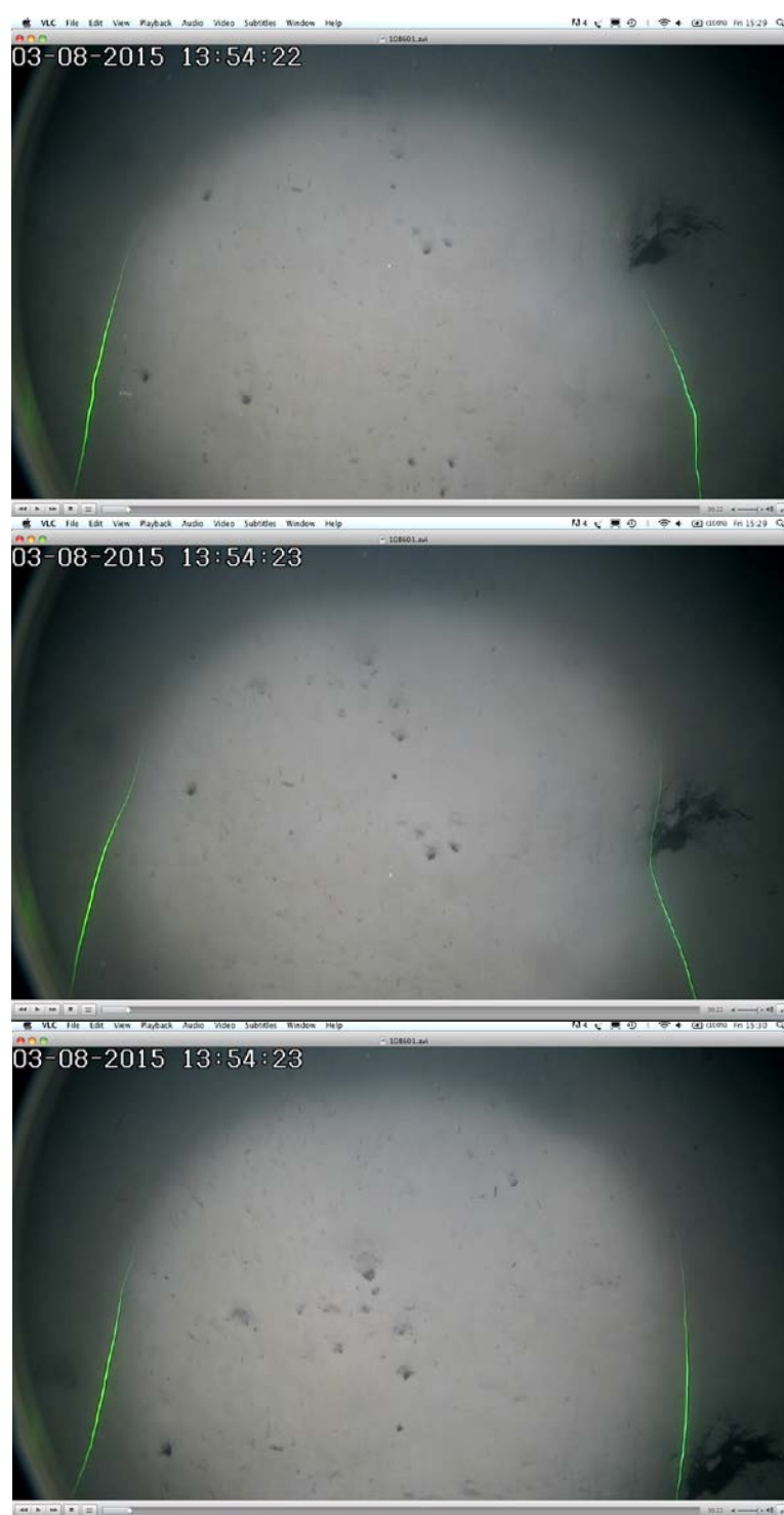
Figure 5.11. FU3-4: Still image of video footage showing the misinterpretation where the stripe laser appears to bend around burrows. In this case the burrow on the right hand side is not counted.
