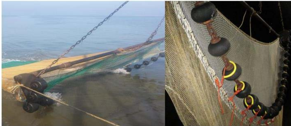
Figure 11.10.2. The Sieve-mat is placed in front of the trawl opening and attached to the footrope.
