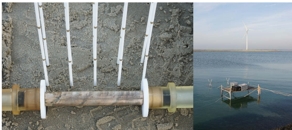
Figure 11.10.7. Left: Field strength probes positioned opposite a conductor. Right: Measurement system at high tide (2 m water height above the electrodes)
