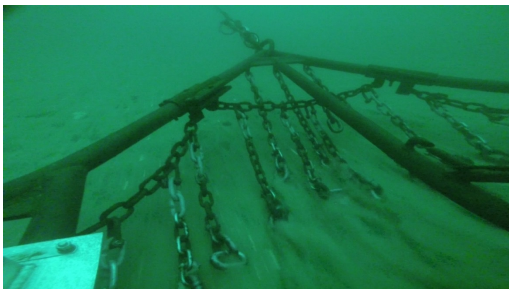
Figure 12.123.1: Still images from GoPro camera attached to dredge frame. Tickler chains making bottom contact during comparison tows.
