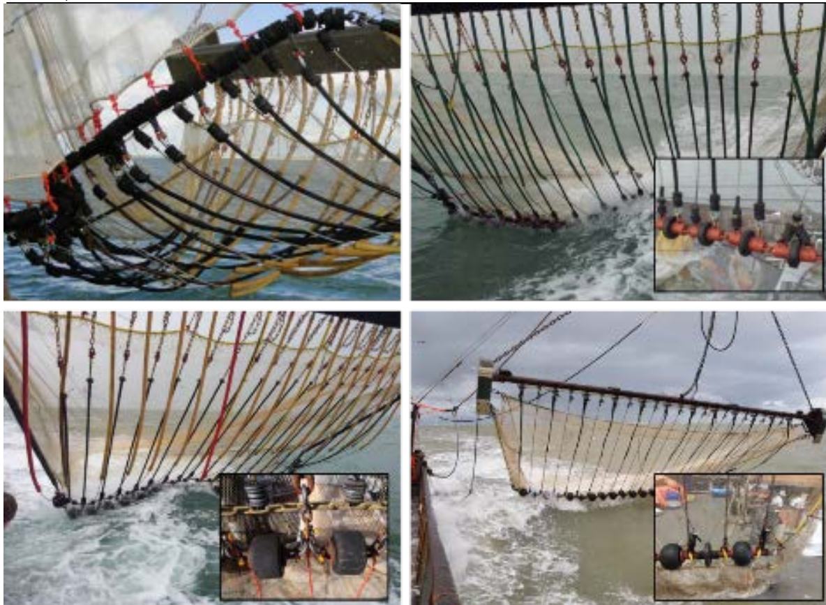
Figure 3.3: Four different ground gear designs tested in a pulse trawl on the Dutch eurocutter TH 10. Each design resulted in different bycatch rates when compared to a standard trawl. Bycatch reduction increased with the size of the escape opening between the seabed and the footrope. Modified from Verschueren et al. (2013).
