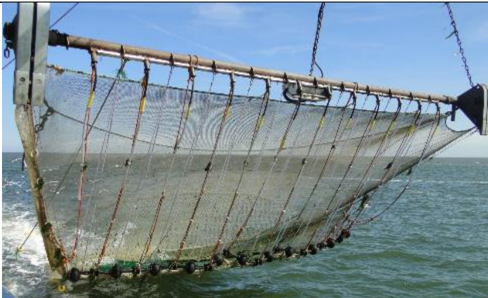
Fig. 2-6 - Image of a pulse trawl design that is being used today on the Dutch Wadden Sea by HA 31. The gear is characterised by the use of a straight, lightweight bobbin rope with 11 ellipsoidal bobbins (instead of 36 bobbins in the previous traditional beam trawls). The pulse generator (central) and the 12 electrodes are attached to the beam.
