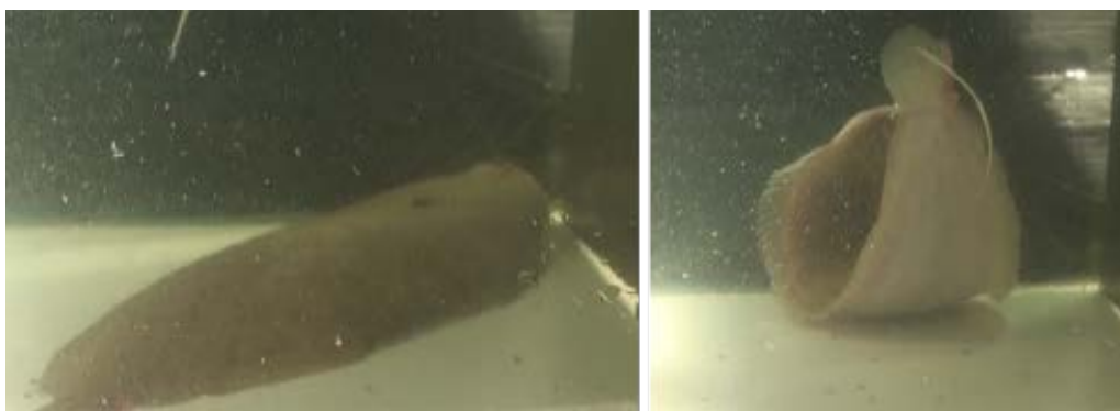
Fig. 2-8 – Dover sole ( Solea solea ) exposed in an aquarium to a pulsed electrical field. As long as the exposure lasts, the muscles are stimulated resulting in continuous spasms. Pulses are bipolar and the pulse frequency varies between 40 and 80 Hz.
