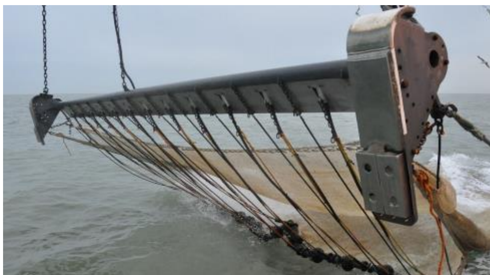
Fig. 2-7 - ILVO's modular pulse fishing system with all electronics built-in a wing
