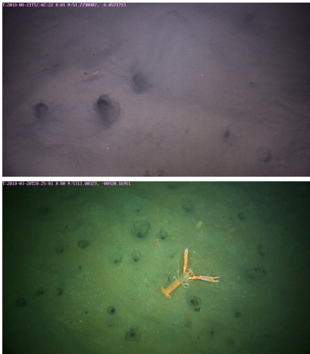
Figure 5.5.1.15. High definition still images from 2018 UWTV survey HD camera system trials. Camera angle 75 degrees, range laser (red dot) and on screen display output (T=Time, R= range laser, N = positional data). The blurred particles in the lower image is marine sediment that is “frozen” when the image is captured. © Marine Institute Ireland.
