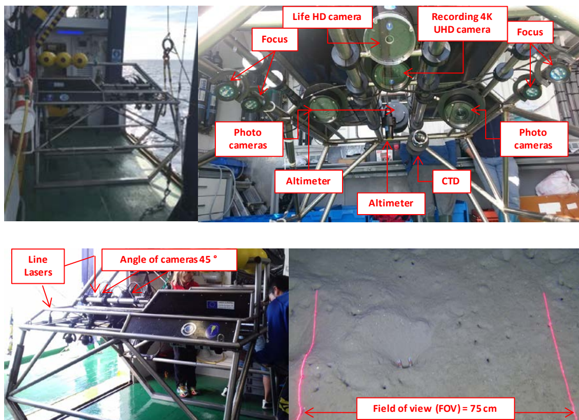
Figure 5.1.6.6. Sledge and equipment use in ISUNEP-CA UWTV survey 2018.
