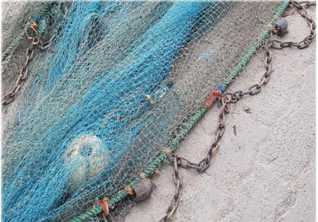
Section of a small shrimp trawl with looped chain groundrope and lead weights on the fishing line (RB Larsen 2019)
