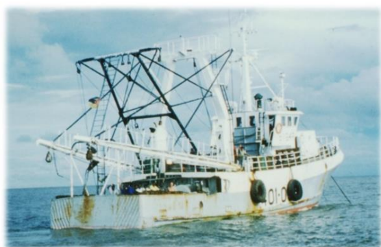
A typical design of a large prawn trawler with outrigger booms for operating twin or quad trawl systems (RB Larsen 1992).
