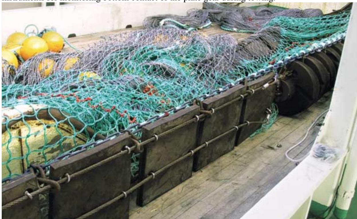
Fig 3.11: The shearing plate gear attached to the fishing line (chain) of a trawl showing port side with square rubber plates and a section of ordinary rockhopper gear behind, i.e. the middle section of the groundrope.
