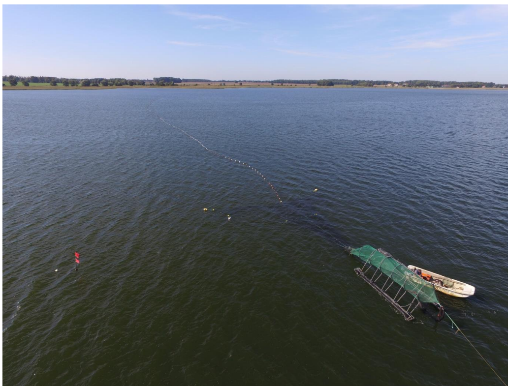
Figure 8.6.9: Pontoon trap in German waters (water depth at position of pontoon trap is approx. 3m)
