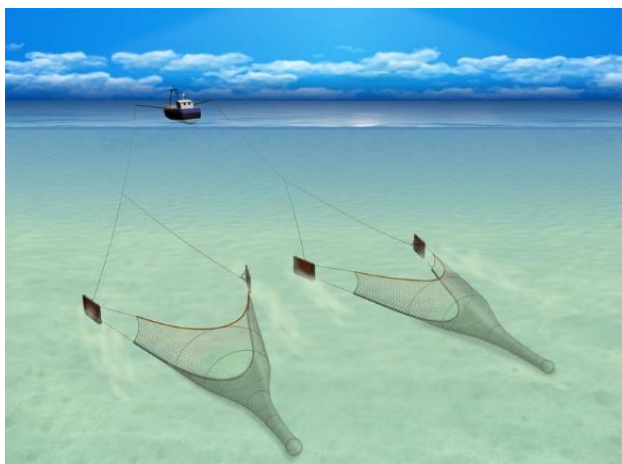
Fig. 4.3.1. An example of a twin trawl rigging operated as single trawl system from each boom (Seafish Assetbank).
