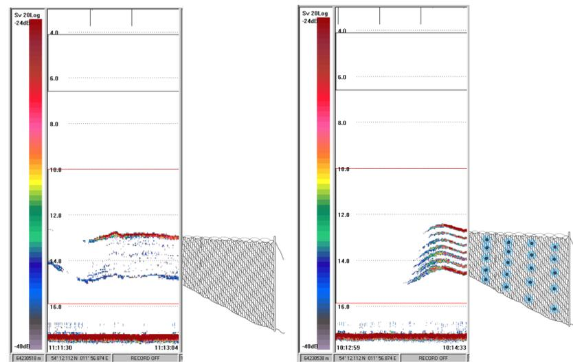
Figure 8. echogram (acoustic image) at 120kHz (echo-locating frequency of harbour porpoises) of a standard gillnet (left) and a gillnet modified with acrylic glass spheres (“pearl net”, right).
