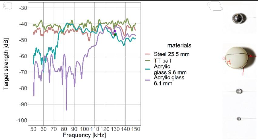
Figure 6. Acoustic reflectivity (Target Strength) of several objects (table tennis ball, steel ball, acrylic glass). The objects have similar echo characteristics between 120 – 150 kHz.
