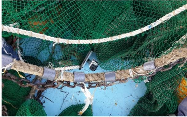
Central part of standard groundgear (above) and modified groundgear (below).
