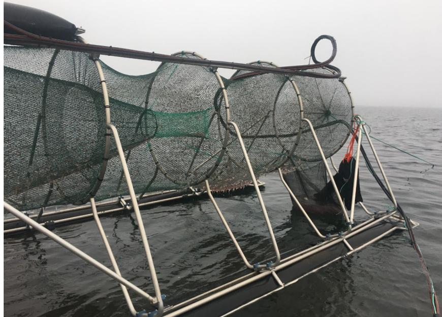
Alternative entrance in pontoon trap chamber. Traditionally strings are used in the chamber entrance. Also, the fish chamber is equipped with hose net for catch collection.
