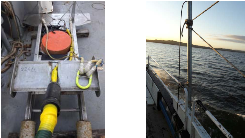
Figure 2.8. Towed-body mounted 38 and 120 kHz transducers and the RV Celtic Voyager , left, and the pole mounted 120 kHz on the FV Ros Ard , right. The 120 kHz echosounder was calibrated in Lough Swilly on 17/12/2019.
