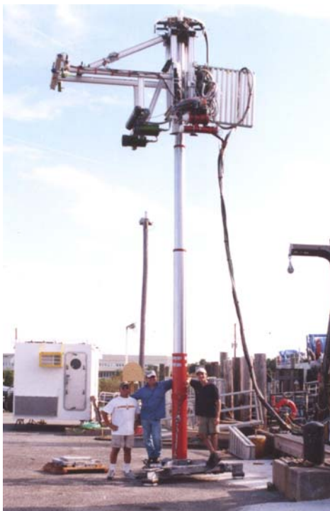
Figure P1. Oceanic Submersible Particle Image Velocimetry System. From “Turbulent stress measurements in the coastal ocean using Particle Image Velocimetry (PIV)” by W. A. M. Nimmo Smith, Thomas Osborn, L. Luznik, W. Zhu, A. Fricova, and J. Katz (Doc P:02).
