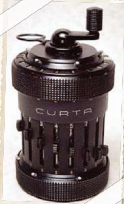
▲ The Curta mechanical rotary calculator was developed by Curt Herzstark while a prisoner in the Buchenwald concentration camp during World War II. It was first marketed in 1948 and was considered the best portable calculator available until rendered obsolete with the introduction of electronic hand calculators in the early 1970s.
