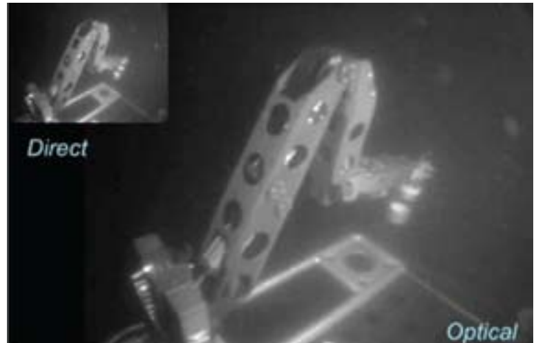
▲ In recent dock trials of the optical modem system, the "Nereus" vehicle performed manipulative tasks while virtually tethered to its surface control station, demonstrating the ability of such a link to support tetherless ROV activities. The image above is a composite of real-time video frame captures showing the direct image (upper left) relayed to the surface via a traditional hard-wire tether compared with the video transmitted wirelessly through water via the optical modem. (Woods Hole Oceanographic Institution.)
