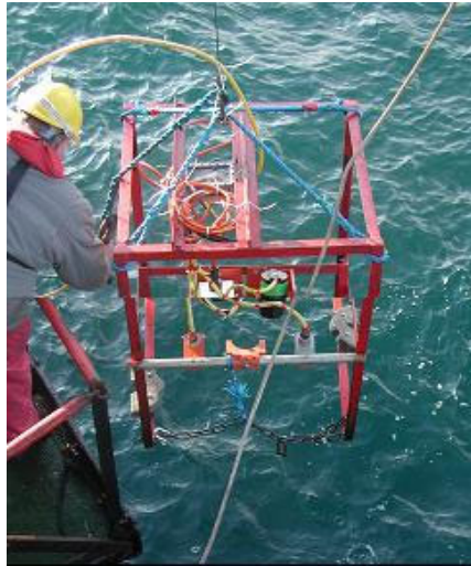
Figure 8.2. Typical drop-down camera frame fitted with an underwater video camera, lights, still camera, and strobe.
