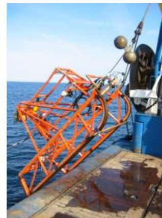
Figure 8.3. A towed platform, typically fitted with an underwater video camera, lights, still camera, and strobe.
