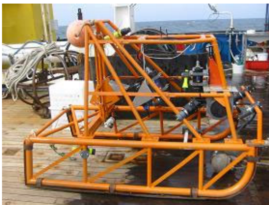
Figure 8.3. A towed platform, typically fitted with an underwater video camera, lights, still camera, and strobe.
