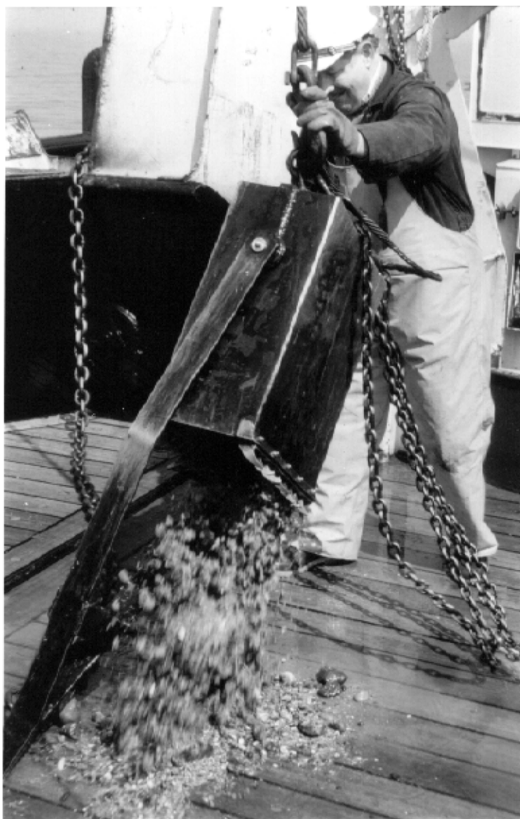
Figure 4.1. Anchor “box” dredge, after Forster (1953).
