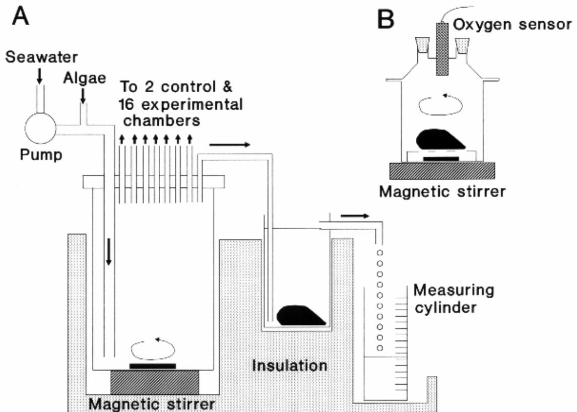
**Figure 1A. Flow-through apparatus for maintaining and feeding of mussels.**
