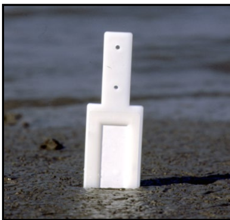
Figure 2. DGT probe inserted in sediment
