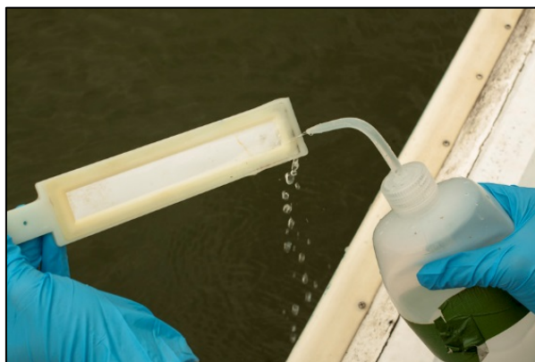
Figure 3. Rinsing of a DGT probe after retrieval.
