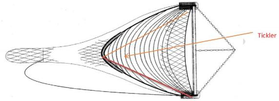
Figure 1 Schematic of traditional beam trawl
