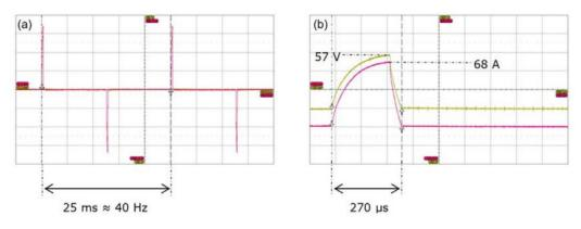
Figure 5 Schematic representation of a pulsed bipolar current (PBC) as used in the pulse fishery for sole (from de Haan *et al.*, 2016).
