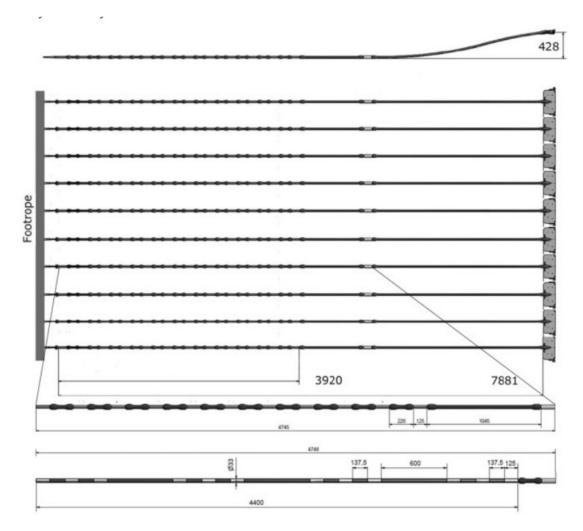
Figure 4 Schematic representation (in mm) of the ten 7.881 m long electrode arrays of a 4.5 m beam-pulse wing used in electrotrawls, targeting common sole with a close-up of two possible electrode array types (from HFK Engineering B.V.). The white or grey conductive parts are made of stainless steel or copper, respectively, and are called electrodes, whereas the longer black parts are non-conductive and called insulators or insulated parts.
