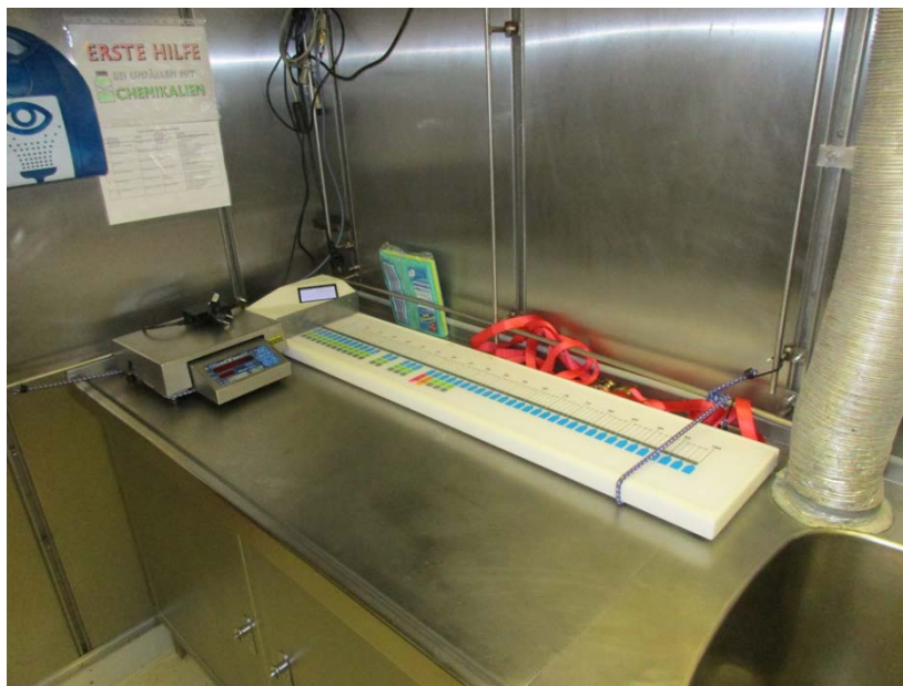
Figure 7.2.2. One of the open source measuring board projects presented at WKSEATEC. openSMB measuring board using linear magnetorestriction sensor and linked to electronic marine scales.
