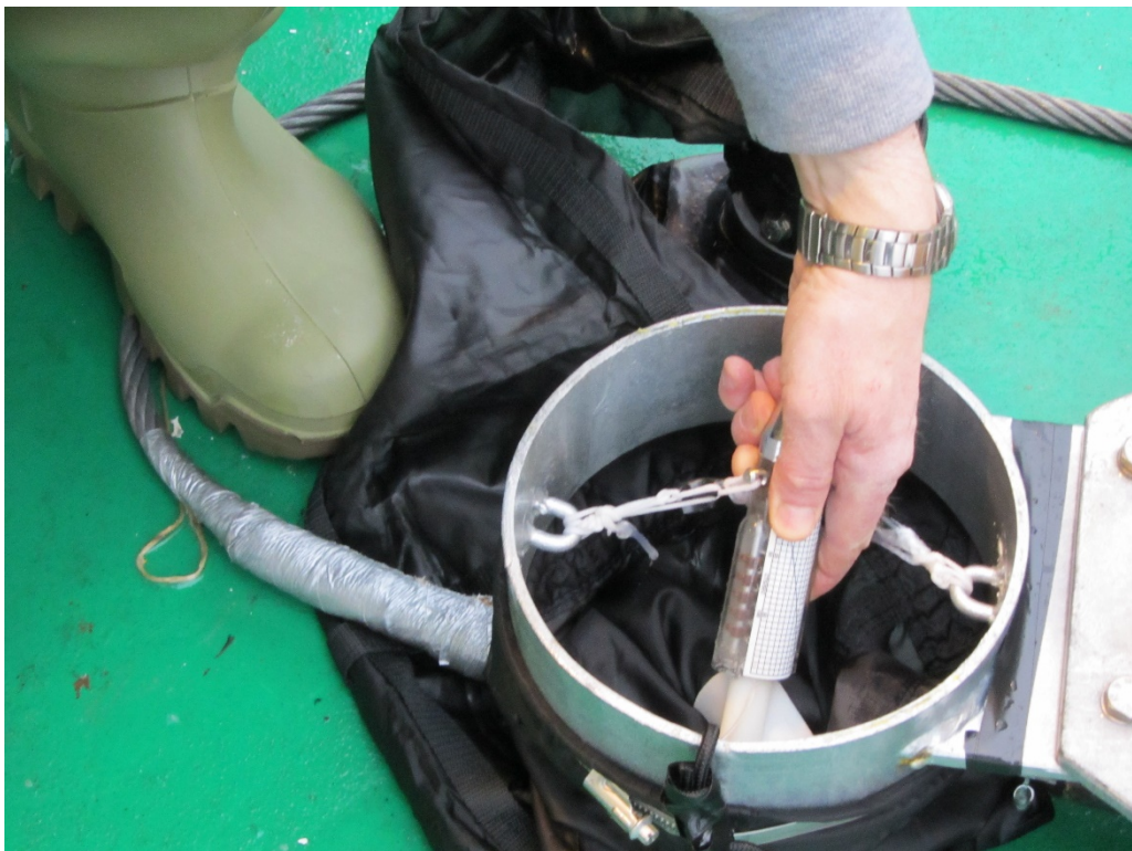
Flowmeter attachment inside MIKeyM ring
