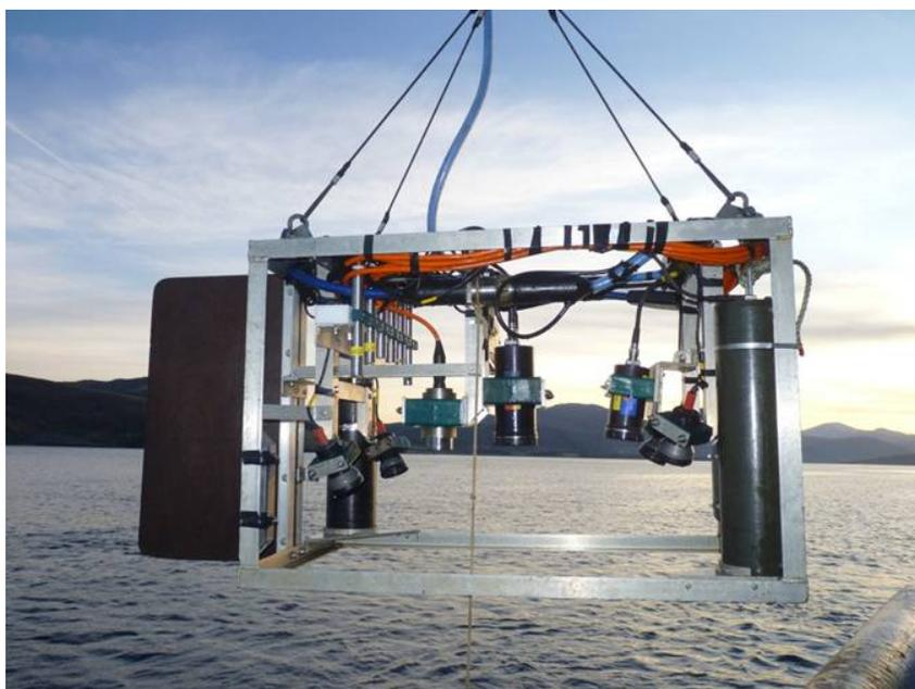
**Figure 2. Image of MSS' suspended drop frame UWTV system used in this survey.**
