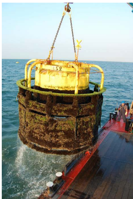
Figure 4.3. Example of a D1 mussel cage.
