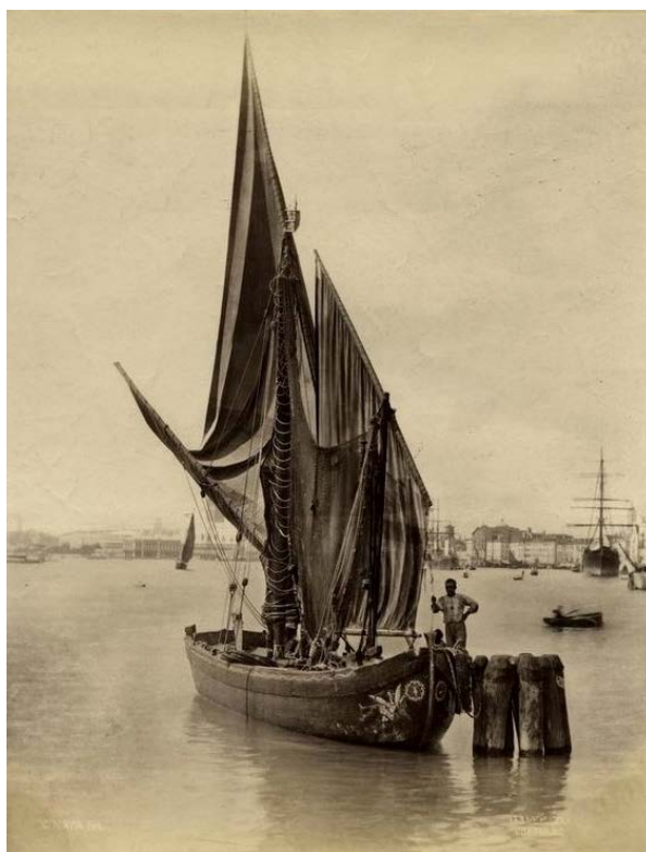
Figure 10. Bragozzo sail trawler in Venice Lagoon, ca. 1880. The net can be seen hanging between the two masts.
