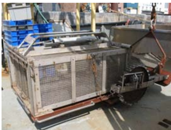
Figure b16. Benthic sledge for shellfish survey in the coastal waters.
