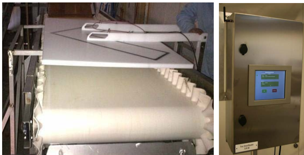
Figure 3.6.2.2.4. RFID antenna (left) and reader system with GPRS in a waterproof locker on the wall (right) that automatically detects RFID tagged fish and updates IMR database over GPRS with necessary data.
