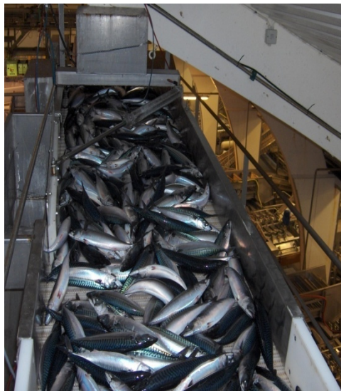
Figure 3.6.2.2.3. Metal detectors with deflector gates used 1986–2010 to recapture mackerel tagged 1977–2009 with internal steel tags.
