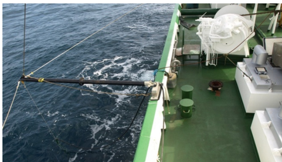
Figure 3. Towing boom c.3m long, with support stays.
