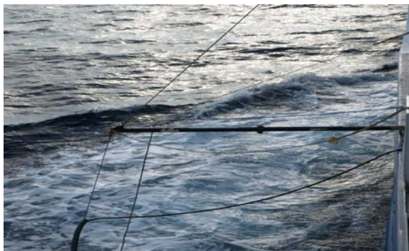
Figure 3. Towing boom c.3m long with support stays.
