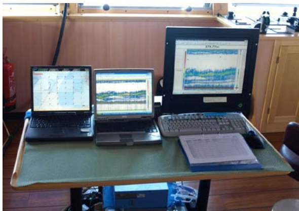
Figure 4. Top side monitoring station located on the bridge. (L-R) Laptop running Sodena© navigation package, second laptop running Echoview© (Live viewing) and EK 60 topside PC unit.
