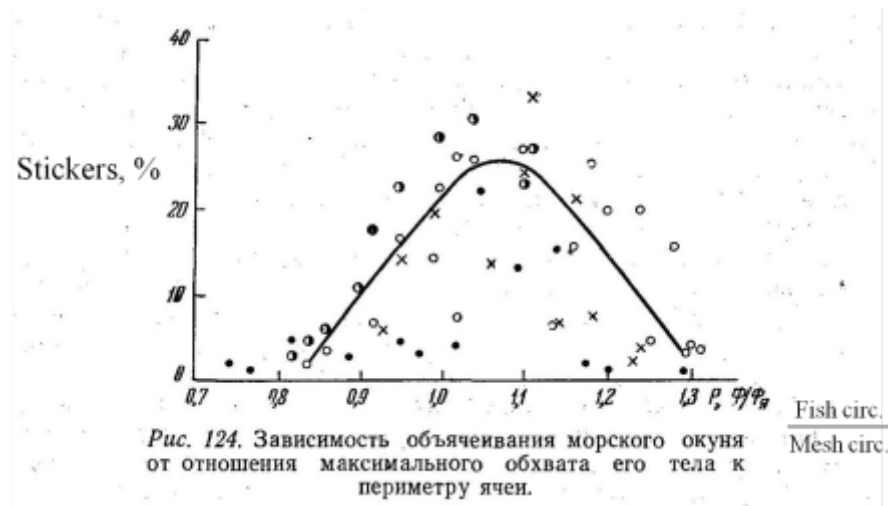
Figure 3. Relationship between redfish stickers and ratio of circumferences of redfish and mesh (Treshev, 1966).
