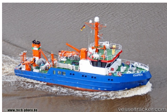
Figure. 3 The new vessel „FFS CLUPEA“ took over the RHLS survey operation in late April 2012. It provides accommodation for 4 scientists, laboratory space and sophisticated means of oceanographic measuring.
