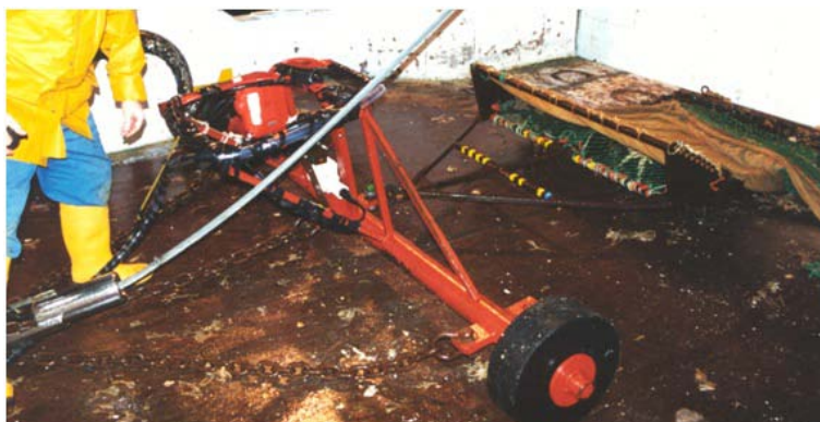
Figure 1. The video dredge system developed by Marine Scotland Science.
