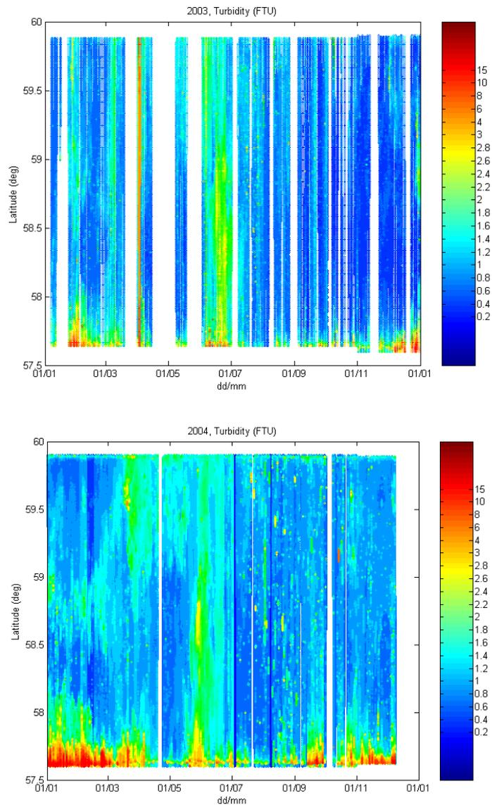
**Figure 6: Plot of turbidity (FTU) for the Skagerrak ferry route from 2003 to 2004**
