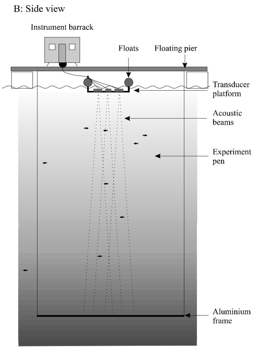
Figure 1. Experimental setup during measurements of cod. Transducer platform not to scale. Experimental pen 12.5 x 12.5 x 21 m.
