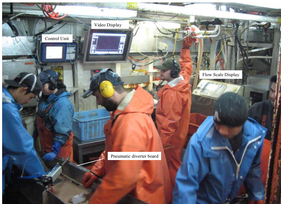
Figure 3. Samplers and sorters working within the sampling station and the equipment layout within the station.
