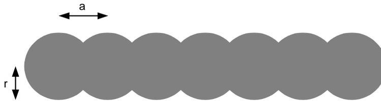
Fig. 2. Idealised footprint of a stack of seven echoes. The ship advances the distance  $a$  between pings and each ping has a footprint of radius  $r$ .
