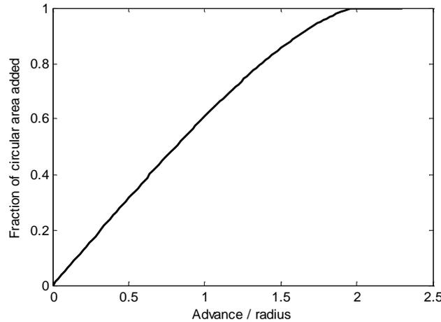
Fig. 3. The fraction,  $\xi$ , of the full circular area that a ping, other than the first one, adds to the area insonified by a stack of pings.
